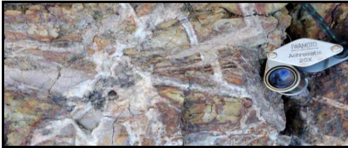
Brecciated ore with fracture filling
